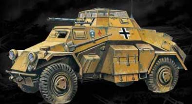
The German Sd. Kfz. 222 was the main light armored vehicle of the German Wehrmacht. This vehicle was built on the Horch 801 chassis.
