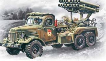
High exploitation qualities of ZiL-157 truck made it an excellent base model for various army vehicles - fuel trucks, command and staff mobile posts, radio and radar stations, medical cars, multiple launch rocket systems.
