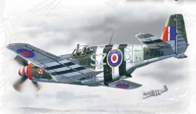
The modification P-51B was built in May 1943. It differed by the installation of potent and high altitude Packard Merlin engine. The airplane Mustang with this engine became one of the fastest fighters in the world. It had huge range, was well armed and armored. Mustangs, produced by a plant in Dallas, were meant as P-51C.
