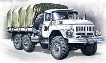
The ZiL-131 6x6 truck with 3,5t capacity replaced in the Soviet army ZiL-157 vehicle. Serial production of ZiL-131 began in 1966 in the Moscow Likhachov automobile factory.
