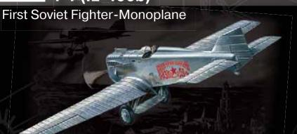
I-1 (IL-400b) was the first fighter created in the USSR and the first airplane designed by N. N. Polikarpov. The unusual distinctive feature of IL-400 in twenties was cantilever monoplane wing design.
