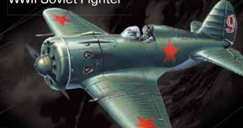
I-16 — the world's first high-speed fighter and the most numerous Soviet aircraft in mid 30s-early 40s period. The cantilever monoplane with retractable chassis I-16 was designed by N. N. Polikarpov in 1933.
