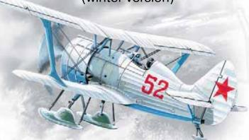
The improved version of I-15 fighter was the I-15bis. Its main differences were "normal" wing centre section and NACA type engine cowling. Serial production of I-15bis began in 1937 and continued to 1939.
