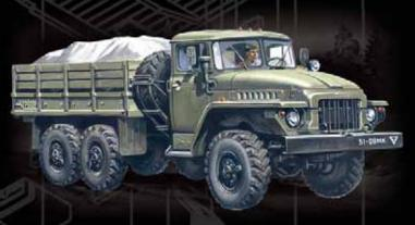
The Ural heavy truck was standard 6x6 wheel vehicle of 5t capacity for the Soviet Army. The modification Ural-375D was produced since 1964 in Miass.
