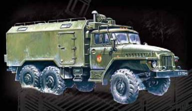
Ural-375 chassis was used as the base for various special vehicles, such as command mobile posts, radio and radar stations, transport and launchers for anti-aircraft missiles, fuel bowsers and multiple launch rocket systems.
