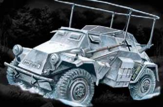
The Sd. Kfz. 261 was another variant of the unarmed radio communication vehicle. Its main difference from the Sd. Kfz. 260 was the type of antenna.
