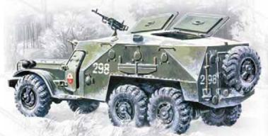
The BTR-152V was adopted as standard APC for Soviet Army in 1958. It was developed on the base of ZiL-157 army truck. The modification BTR-152K had hull roof plate.
